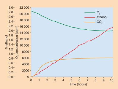
Figure 5.27 Output from a fermenter
