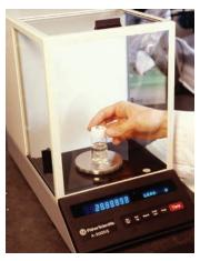
A B Figure 1.10A This balance is accurate to 0.01 g
