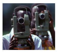
**Figure 1.27** A theodolite – this is used to measure the height of trees or of slopes in the area
