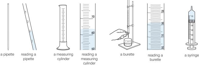
**Figure 1.6** Different measuring apparatus
