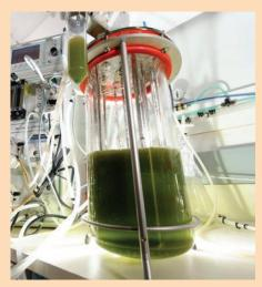
**Figure 5.26** A fermenter that monitors changes electronically
