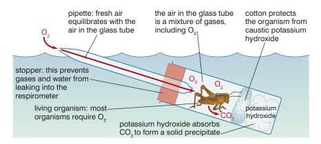
Figure 5.16 A basic respirometer
