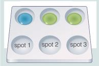
*Figure 1.7 Using a standard to compare colour changes*
